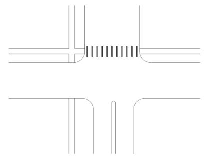
In order to form a continuous pedestrian system, the addition or relocation of sidewalk segments may be required:
