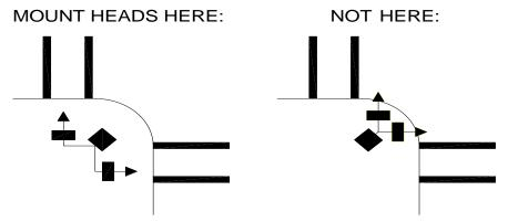
Some states require the designer to determine the number and size of conductors required to serve all of the vehicular and pedestrian heads at an intersection. The designer does this by completing a series of voltage drop calculations. A detailed wiring diagram is then provided as part of the plan set. Other states use standard specifications to identify the number of conductors required for a given situation.
