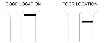
A stop line location close to the end of a median nose is a more natural stopping position than one some distance from the median nose. Not locating stop lines in their natural position will result in some drivers pulling past the stop line.
