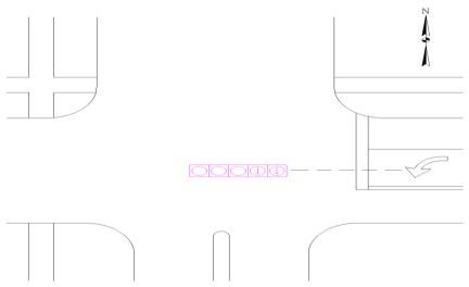
Note that, if the 5-section cluster is replaced by a straight 5-section head or a 4-section head, then an additional 3-section head will be needed in the east approach thru lane to maintain the two required indications for the thru movement.
