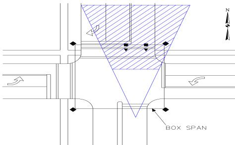
Concrete or wooden strain poles configured as a box span:
