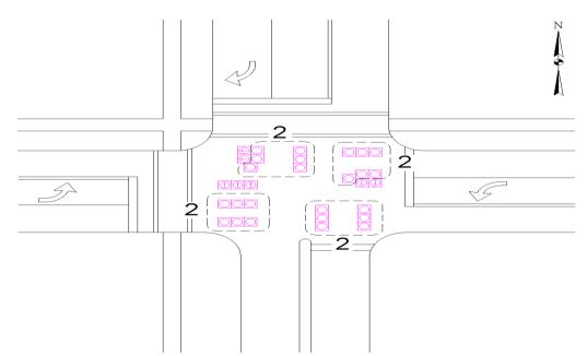
Note that all thru movements in this example are controlled by at least two signal indications:
