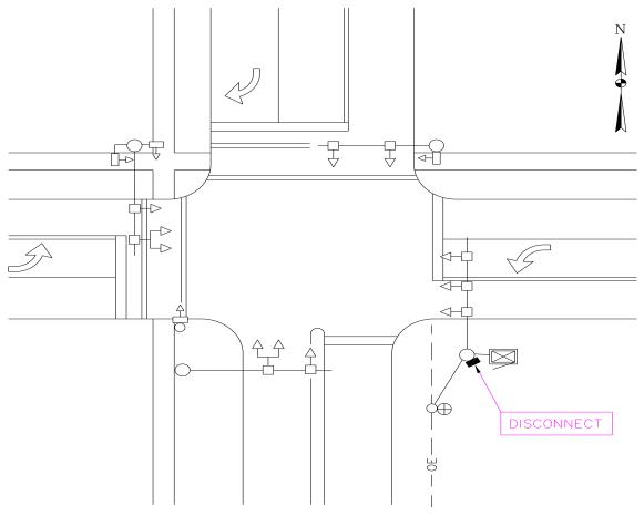
Locating the disconnect on the controller cabinet is not considered good practice since, if the cabinet is leveled by a car, then it will not be possible to shut off the live wires without getting the electric company involved. The wire that goes from the power source to the cabinet via the disconnect is usually referred to as the "electric service wire".
