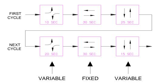
During a given time of the day, such as the AM rush hour, the green time provided to the side street phases and the main street left turn phases under semi-actuated control can increase or decrease depending on the amount of vehicular demand, but the green time provided to the main street through
