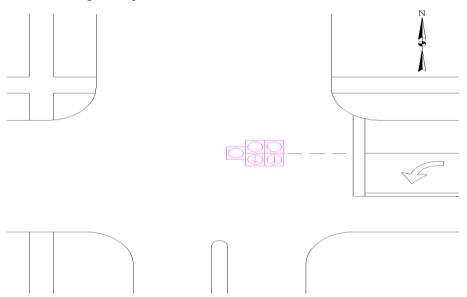
When a "straight 5" signal head or a 4-section FYA head is used the head is typically centered in the left turn lane.
