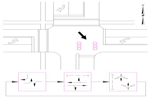
The phasing diagram at the bottom of these drawings depicts how the signal will operate. First the major street turns will be given the green indication:
