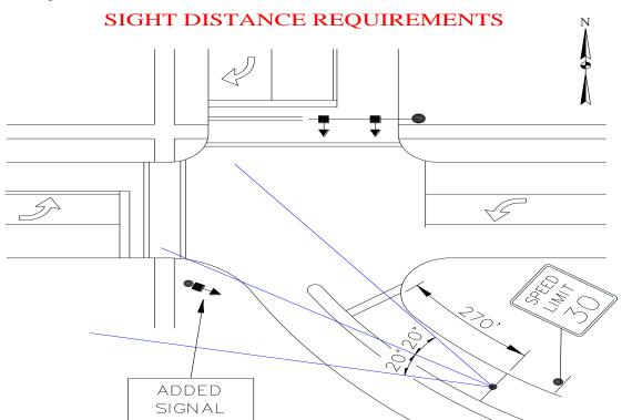
traffic. If the previous example is modified to include a severely curved approach, then at least one more signal head would be added:
