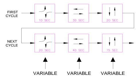
During a given time of the day, such as the AM rush hour, the green time provided to each phase can increase or decrease depending on the amount of vehicular demand. Vehicle demand at a fully-actuated signal is monitored by detection devices located on the various approaches to the intersection.
